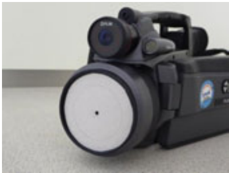
Figure 20: Pinhole in piece of cardboard in front of the camera lens
