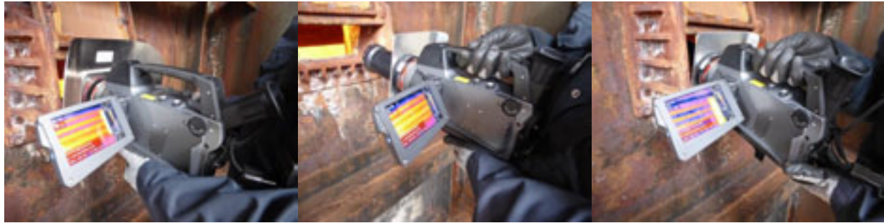
Figure 17: The camera looking through a peephole with (right) and without (left) the lens extender
